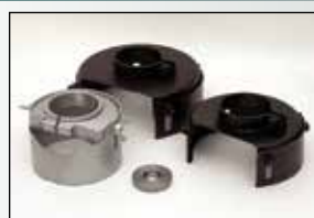
Cup wheel guard and flange for mounting 4" - 6" Type 11 cup wheels on 7" - 9" angle grinders Guards: 655174000 - 4"/5", 655178000 - 6". Mounting flange US90357006
